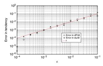
**Figure 15.** Control of tendency error in the inertia–gravity wave regime. The thresholds for pressure and velocity are respectively  $\varepsilon_P = c U \varepsilon^{3/2}$  and  $\varepsilon_u = U \varepsilon^{3/2}$ , to ensure that the error in the tendencies  $\partial_t p$  and  $\partial_t \mathbf{u}$  are  $O(\varepsilon)$ . This figure is available in colour online at wileyonlinelibrary.com/journal/qj
