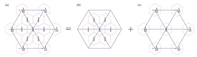
**Figure 8.** Decomposition of (a) the pressure restriction operator  $R_p^i$  into a sum of (b) an area-weighted restriction operator  $R_0^i$  and (c) a remainder  $\delta R_p^i$ . The remainder is proportional to the seven-point Laplacian on the coarse grid. This figure is available in colour online at wileyonlinelibrary.com/journal/qj
