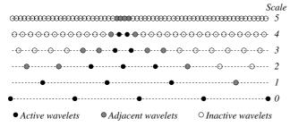
**Figure 11.** One-dimensional example showing adjacent wavelets in position and scale that are added to the grid of active wavelets to account for the change in the solution over one time step.
