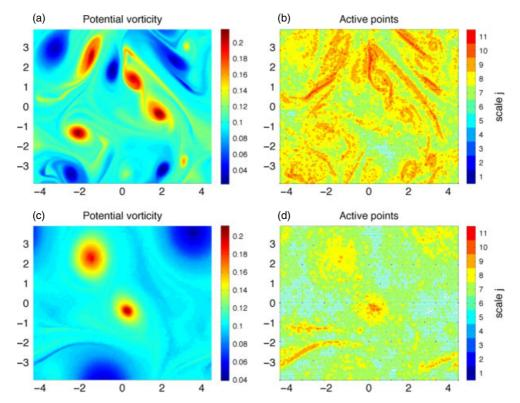
**Figure 22.** (a, c) Potential vorticity and (b, d) adapted grids for decaying quasi-geostrophic turbulence computed with tolerance  $\varepsilon = 0.15$  at (a, b) an intermediate time (t = 39.8) and (c, d) a late (t = 74.8) time. This figure is available in colour online at wileyonlinelibrary.com/journal/qj
