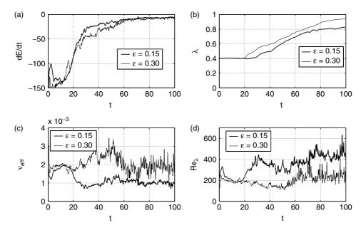
Figure 26. Dynamical quantities compared for turbulence simulations with tolerances  $\varepsilon = 0.3$  and  $\varepsilon = 0.15$ : (a) energy decay dE/dt, (b) Taylor scale  $\lambda$ , (c) the effective viscosity  $\nu_{\rm eff}$ , and (d) the effective Taylor Reynolds number  $Re_{\lambda}$ . The effective Reynolds number appears to be roughly inversely proportional to the tolerance after the initial laminar period.
