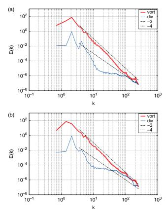
**Figure 24.** Vortical and divergent parts of the energy spectrum for the decaying shallow-water turbulence simulations with tolerances (a)  $\varepsilon=0.15$  at t=25.03, and (b)  $\varepsilon=0.30$  at t=21.80. Note that the vortical part of the two spectra are very similar, while the divergent part of the  $\varepsilon=0.15$  spectrum has less energy at intermediate and small scales. This figure is available in colour online at wileyonlinelibrary.com/journal/qj
