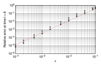
**Figure 17.** Accumulated time integration errors at t=8 for the linear gravity wave case as a function of tolerance  $\varepsilon$ :  $L^1$  error  $(\circ)$ ,  $L^2$  error  $(\Box)$ ,  $L^\infty$  error  $(\diamond)$ . Errors in p are indicated by open symbols and errors in  $\mathbf u$  by filled symbols. The straight line shows a  $\varepsilon^{3/2}$  scaling. This figure is available in colour online at wileyonlinelibrary.com/journal/qj
